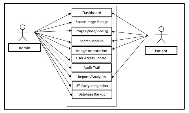
The image shown above is the Use Case Diagram of the system entitled X-Ray Results Image Archiving System. The system has two user sides, the Admin and the Patients. The admin can access the entire core modules of the system while the Patient can access the Dashboard, Image Uploading/Viewing, Search Module, Image Annotation and Reports/Analytics.
